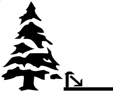
Low light fixture illuminates walk. Vegetation is used to shield light from adjacent properties.
